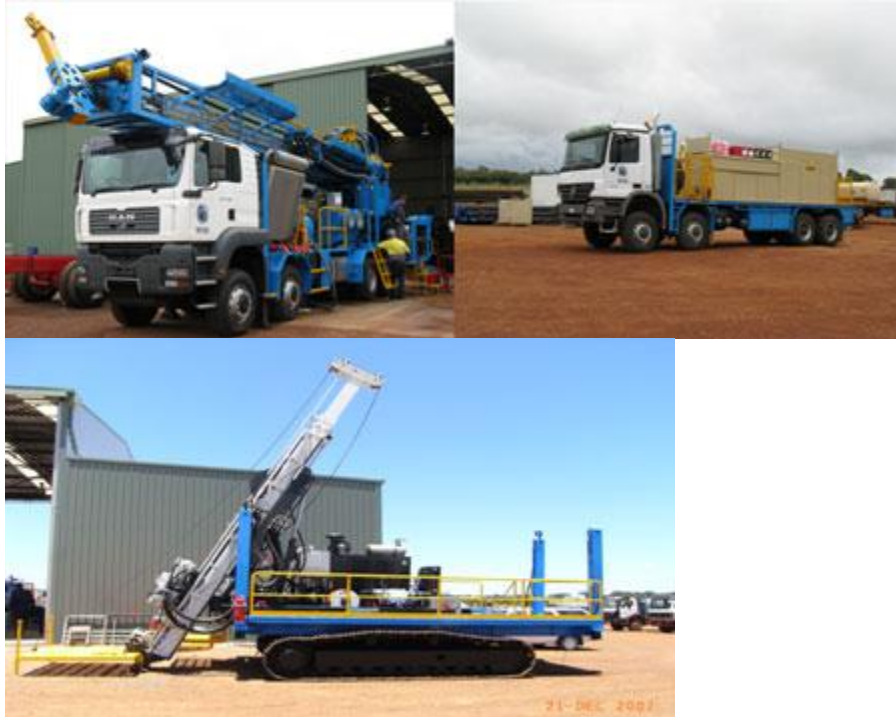
CME 75 HT/Angle Hollow-stem Auger Drill Rig, truck and trailer
